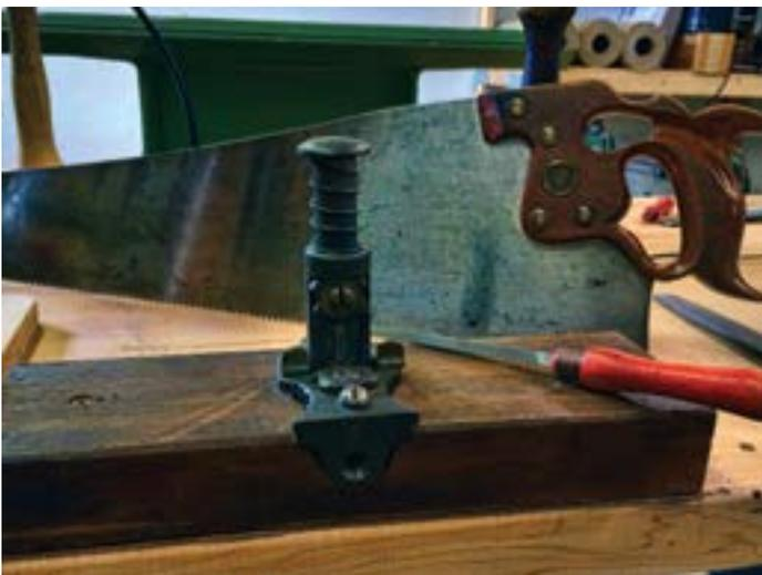
Disston Star hammer saw set, patented 1876
