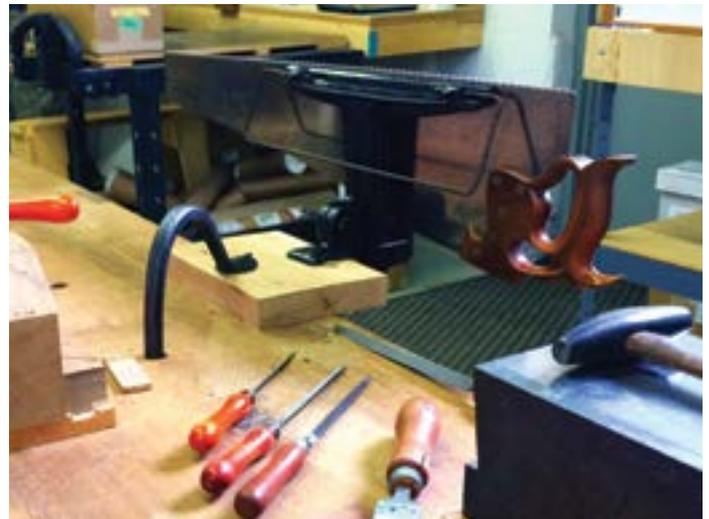
Disston saw sharpening vise No.3D
