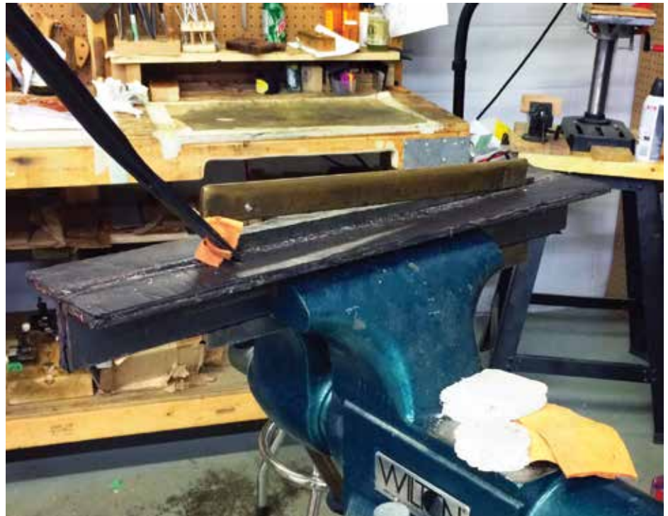
Raising the saw back to separate the handle, back and fasteners
