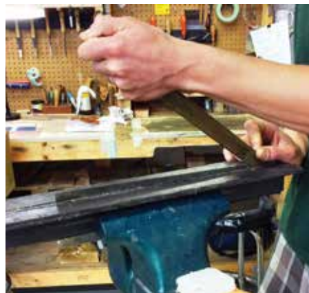
Apply a penetrating oil along the underside of the saw back
