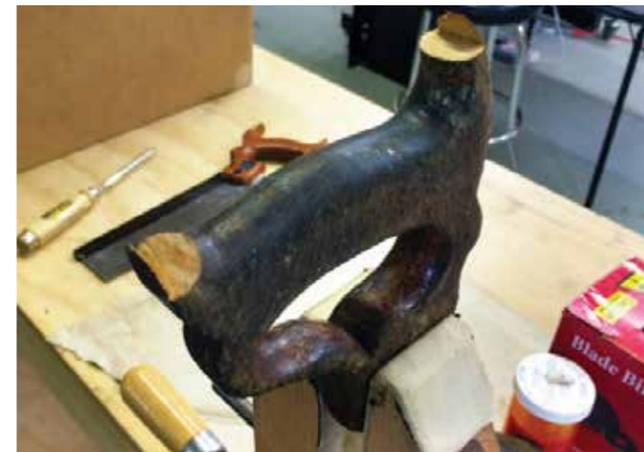
Cinch your handle in a wooden clamp and cut a 90° notch along the damage
