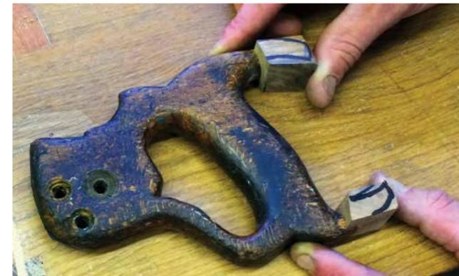
Trace out the horn outline on your graft wood and cut the squares proud of the trace for length, thickness and width
