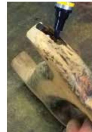
Using a stain marking pen to blend in the grafted wood with the original wood
