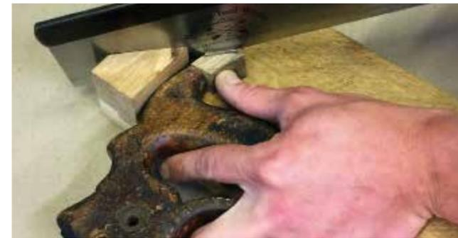
Secure your handle onto a bench hook or clamp and literally saw off the big chunks to rough form
